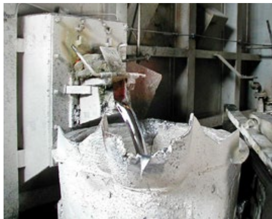
More lightness: In 1998 Zehnder bought the traditional Italian company Faral, which manufactured radiators from aluminium. In the picture, melted aluminium flows into the container, which is then taken to the die-casting machines.
