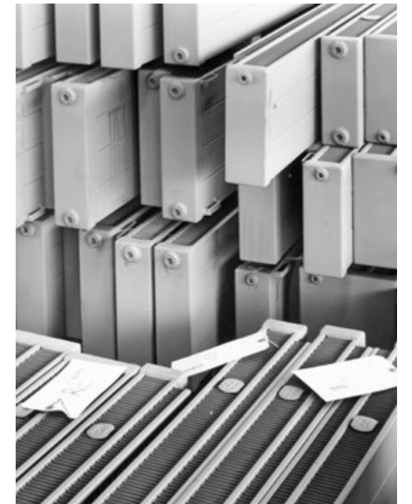
Zehnder convectors are radiators of low height (7 to 35 cm). Between the water-carrying flat tubes, fins are spot-welded to increase the surface area, which causes convection (chimney effect) of the heated air.
