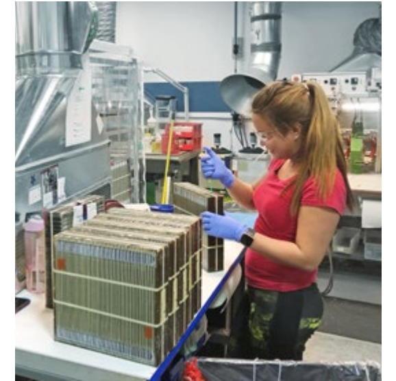
An employee of dPoint in Vancouver, Canada, during the assembly of an enthalpy exchanger. These increase the durability and efficiency of fuel cells - a market with high future potential.
